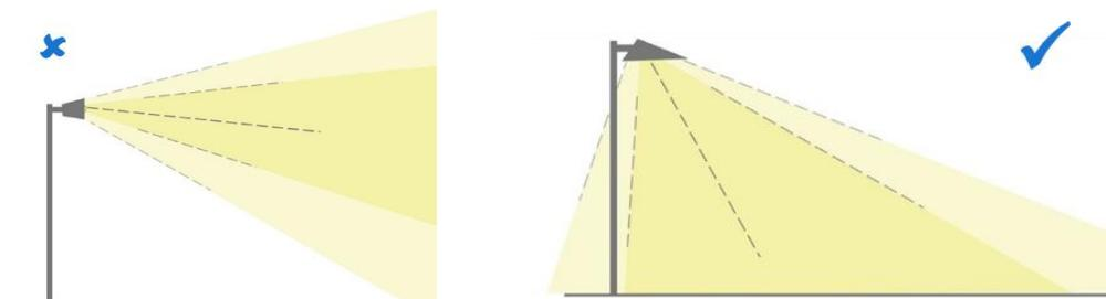
Figure 13: Appropriate floodlighting design includes use of an asymmetric beam
