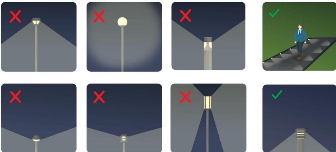
Figure 9: Examples of bad and good walkway lighting
