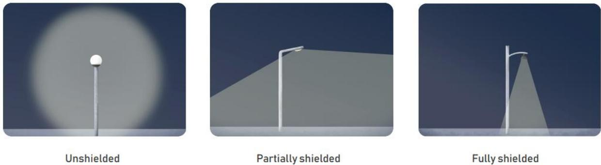
Figure 5: Shielding characteristics of light fittings
