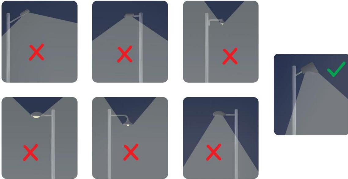
Figure 8: Examples of bad and good pole lighting
