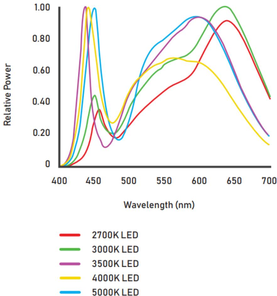
Figure 14: Variation in blue content, (~450 nm peak) as a function of colour temperature, in “standard” LED lights. Lights with the least amount of blue light are recommended. (Source; with permission of Ian Ashdown)
