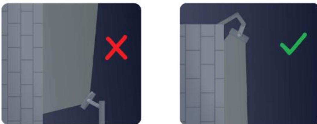
Figure 4: Examples of bad and good aiming angle for a building facade
